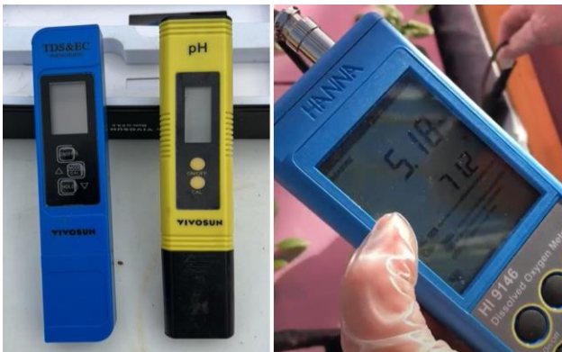
Figure 14. EC and pH meters (left) and DO meter (right). (Toni Sperry, Virginia Tech)
