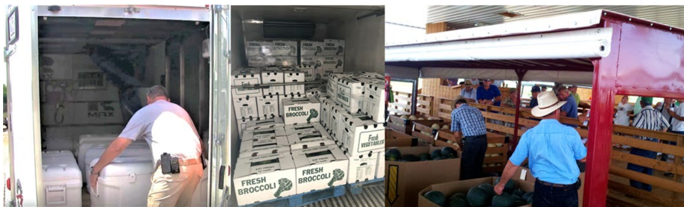
Figure 10. Examples of transport vehicles from left to right: chest freezers containing lettuce being placed into a small, refrigerated trailer equipped with a CoolBot™ device; boxed broccoli stacked on pallets inside a refrigerated truck; melons in bulk bins that have been transported to nearby produce auction using a fully covered trailer with roll down sides to protect from contamination. (Amber Vallotton, Virginia Cooperative Extension, except for center photo by Justin Light)
