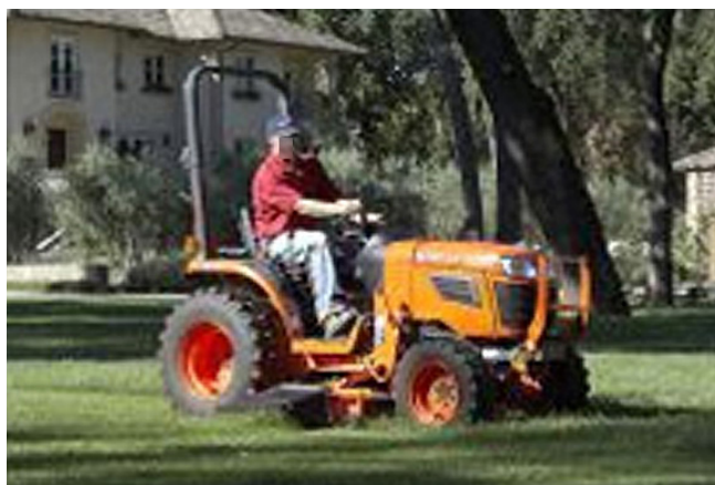
Mower with rollover protection structures.
