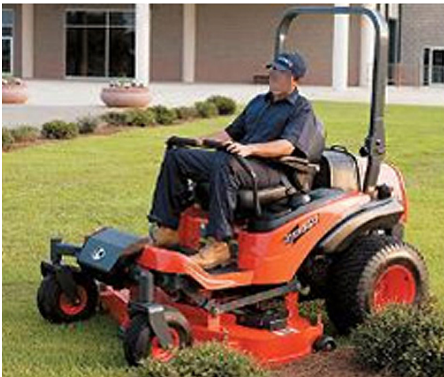
Suspended mower deck with parallel links.
