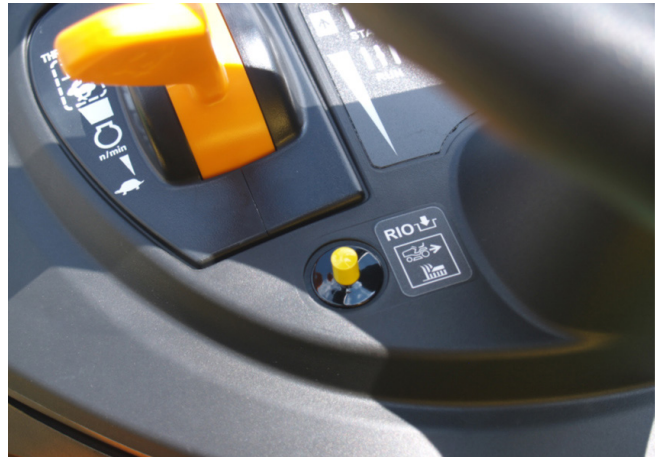
The RIO button must be engaged to reverse the mower with the mower deck running.
