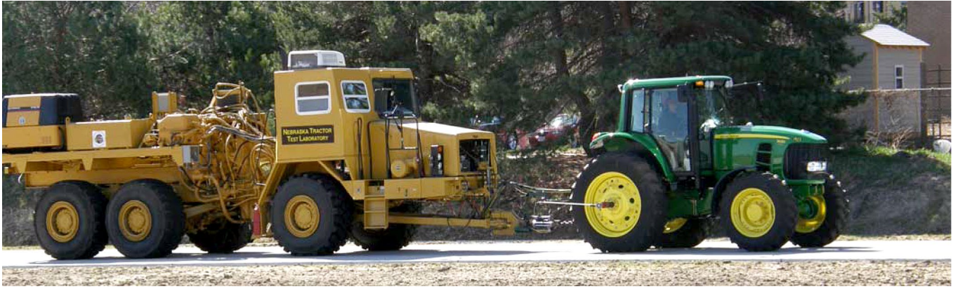
Figure 3. A tractor running on the test course. The drawbar performance test is being performed.
