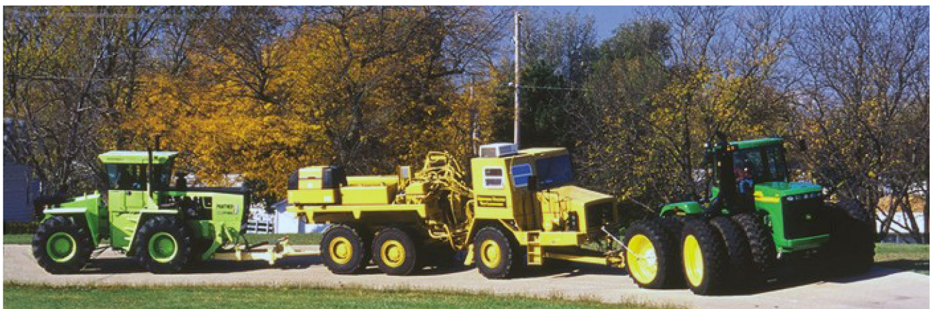
Figure 2. The lead tractor is being tested on the track during drawbar performance tests. The two vehicles in tow are load units.
