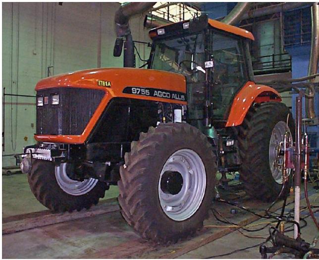
Figure 1. A tractor being tested on the PTO dynamometer. The test apparatus in the foreground is measuring fuel flow.
